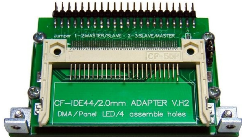
Adapter to convert IDE44 connection to Compact Flash (shown attached to right-angle mounting panel)
